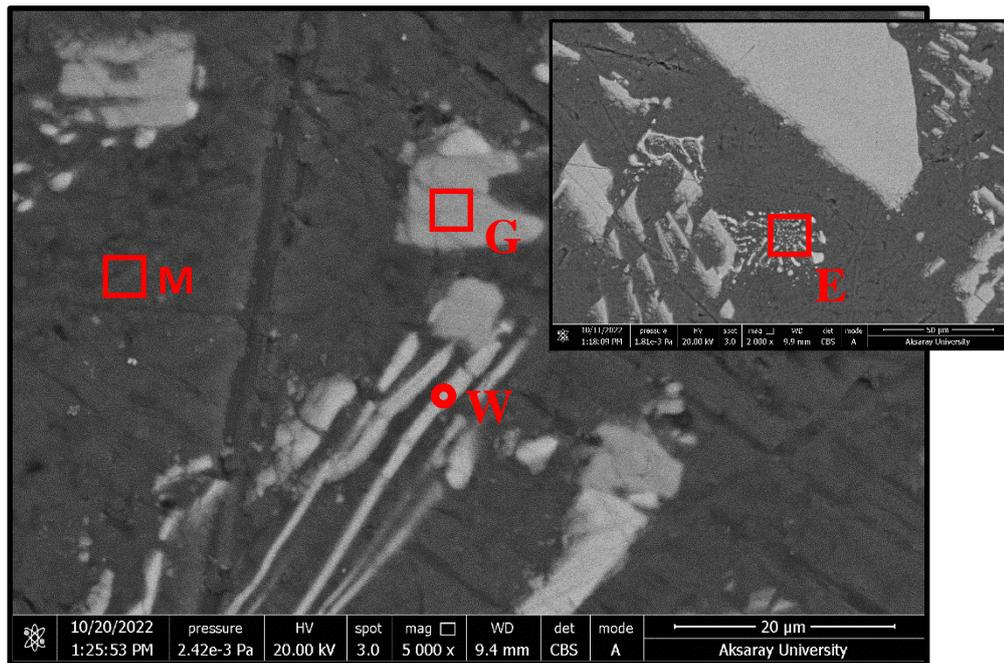
**Figure 2.** SEM image of longitudinal section of non-heat-treated Al-Ni-Mn alloy and, marked phase areas (M: Matrix phase, G: Gray phase, W: White phase, E: Eutectic area).
