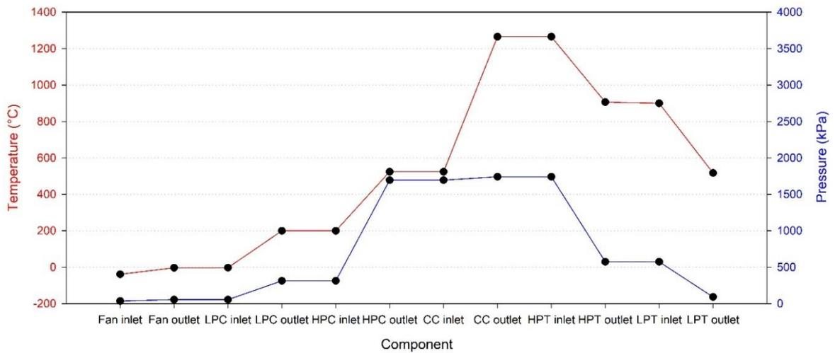
**Figure 3.** Temperature and pressure values of the components
