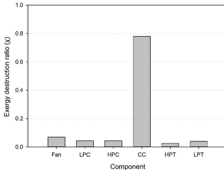
**Figure 6.** Exergy destruction ratios of the components
