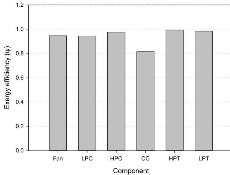
**Figure 4.** Exergy efficiencies of the components
