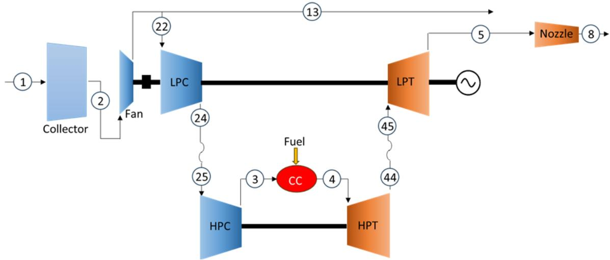
Thermodynamic schematic of the modelled engine
