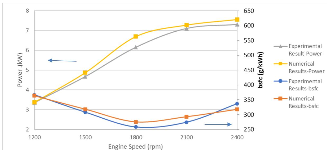
**Figure 3.** Power and specific fuel consumption validation graphs
