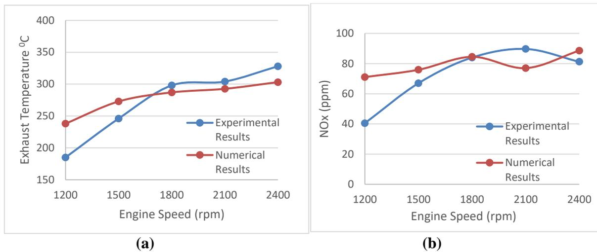
Figure 4. Exhaust a) gas temperature and b) NOx emissions
