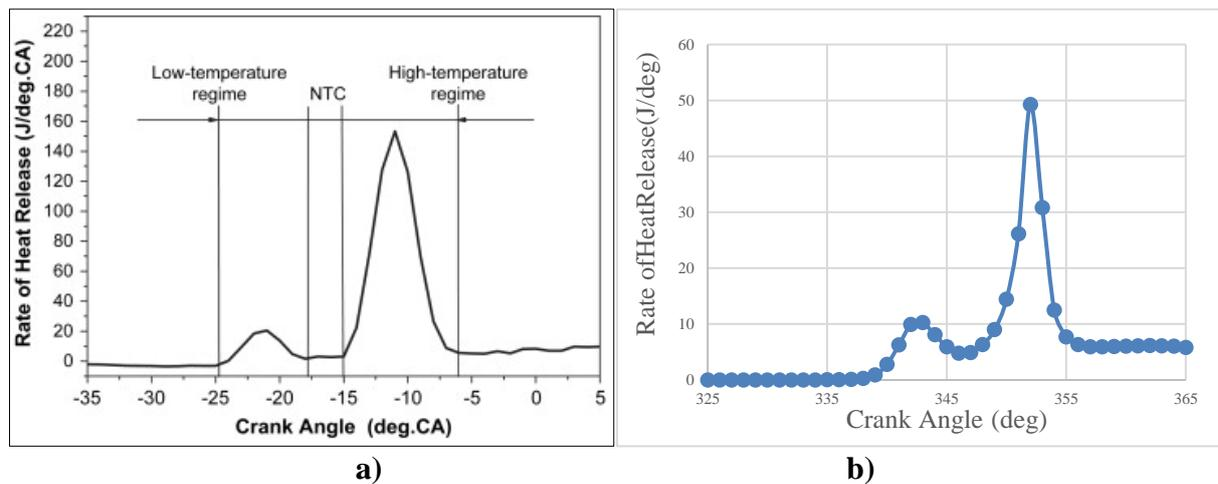
**Figure 8.** Heat Release Curve a) Typical curve for HCCI combustion with n-heptane [28] b) obtained from the model for 1200 rpm,  $P_{in}=0.95$  bar  $T_{in}=20^{\circ}\text{C}$ ,  $AFR=45$
