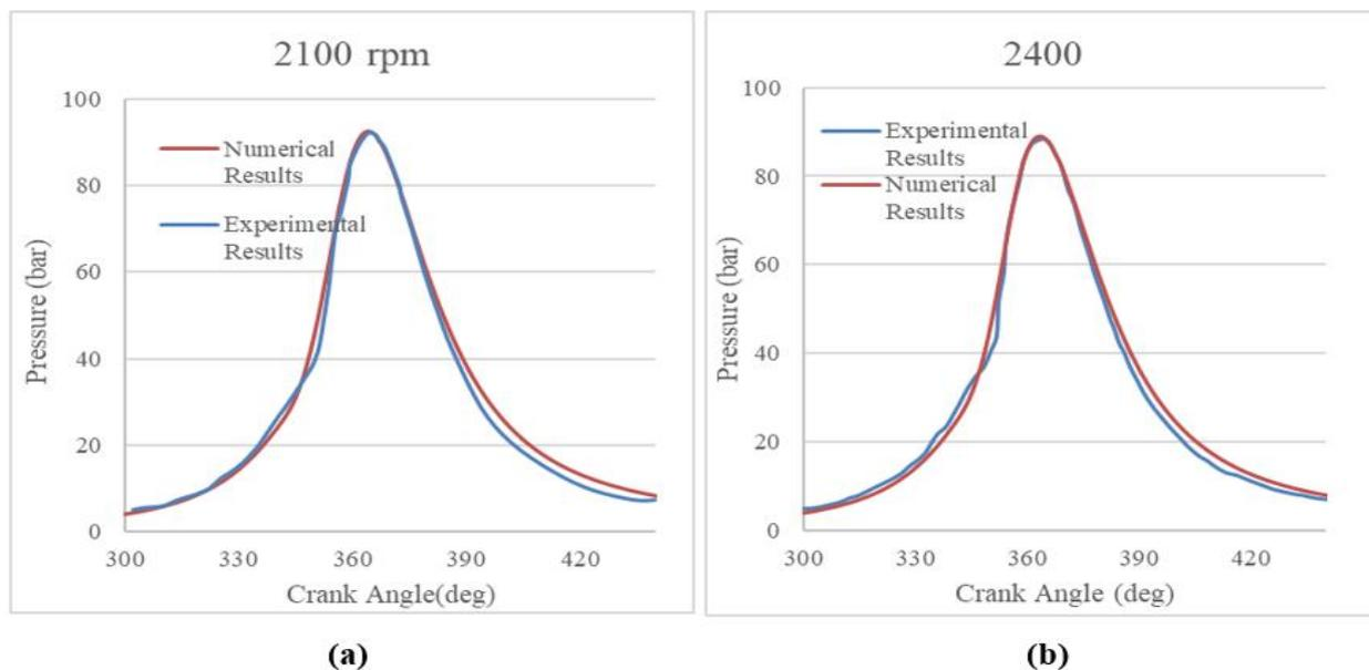
Figure 7. In-cylinder pressure at a) 2100 and b) 2400rpm
