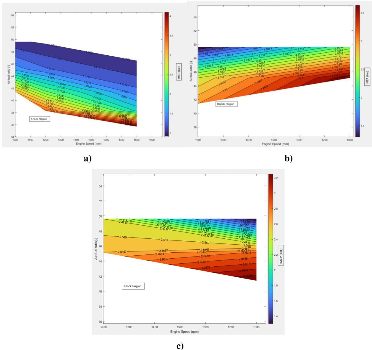
**Figure 13.** Inlet air temperature effect on HCCI operating range and IMEP ( $P_{in}=0.95$  bar CR=15) a)  $T_{in}=20^{\circ}\text{C}$  b)  $T_{in}=40^{\circ}\text{C}$  c)  $60^{\circ}\text{C}$
