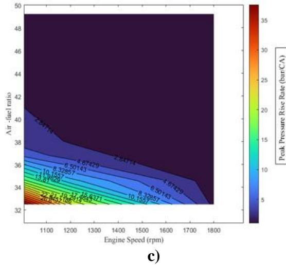
**Figure 9.** Compression ratio effect on HCCI operating range and peak pressure rise rate (Tin=20°C Pin=0.95 bar) a) 17.5 b) 15 c) 13
