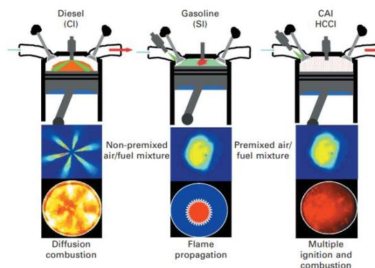
**Figure 1.** Three combustion modes [7]
