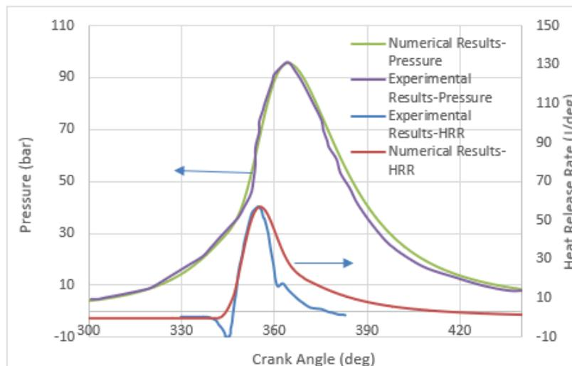
Figure 5. In-cylinder pressure and HRR at 1800 rpm
