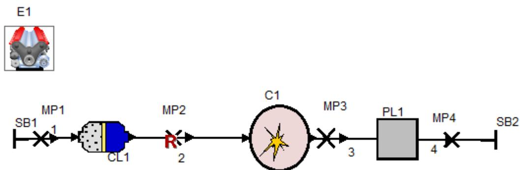
**Figure 2.** AVL Boost image of modeled one-cylinder diesel engine.
